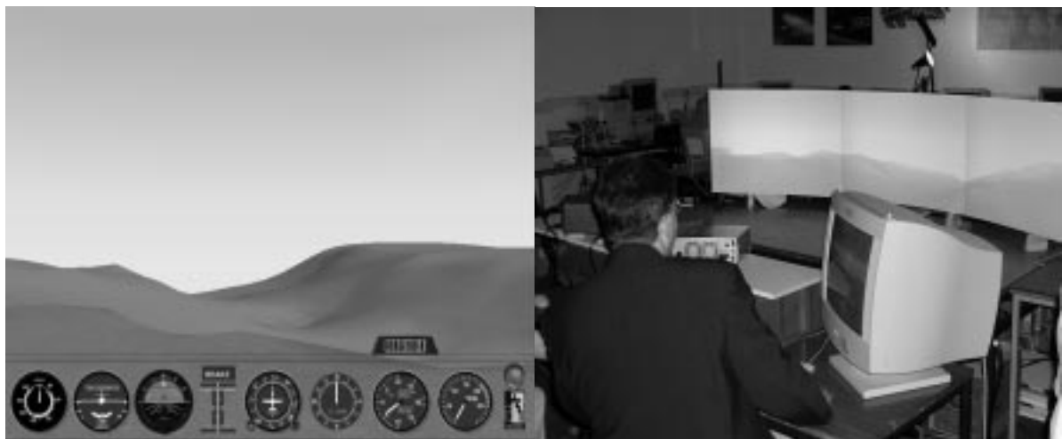
Fig 1 - FlightGear simulator with Martian terrain and multi-screen capability
